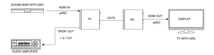
NOTE: In eARC mode the SPDIF output only supports up to 5.1 CH audio.
