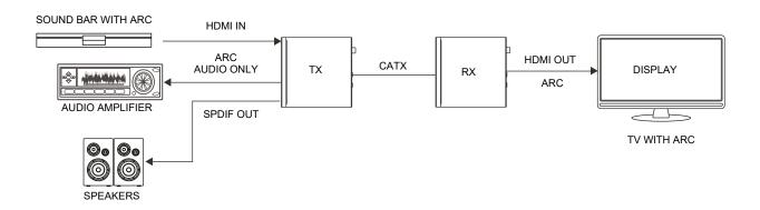
**Scenario 4:** Set the Extender to ARC Mode. Then switch the LOOP OUT/AUDIO ONLY switch to the left, the HDMI OUT port of the transmitter is set to LOOP OUT.
