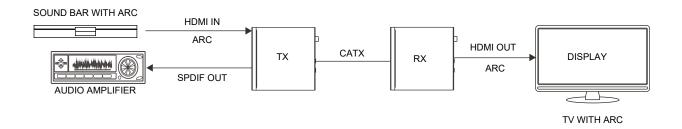
**Scenario 5:** Set the Extender to eARC Mode. Then switch the LOOP OUT/AUDIO ONLY switch to the right, the HDMI OUT port of the transmitter is set to AUDIO ONLY.
