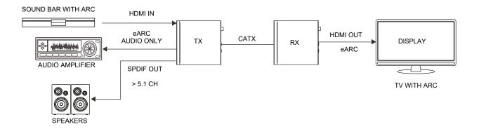
**Scenario 6:** Set the Extender to eARC Mode. Then switch the LOOP OUT/AUDIO ONLY switch to the left, the HDMI OUT port of the transmitter is set to LOOP OUT.
