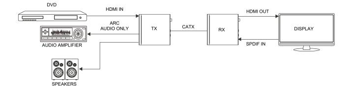
**Scenario 2:** Set the Extender to SPDIF Mode. Then switch the LOOP OUT/AUDIO ONLY switch to the left, the HDMI OUT port of the transmitter is set to LOOP OUT.
