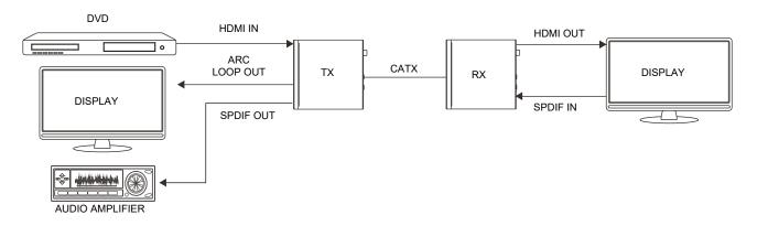
**Scenario 3:** Set the Extender to ARC Mode. Then switch the LOOP OUT/AUDIO ONLY switch to the right, the HDMI OUT port of the transmitter is set to AUDIO ONLY.
